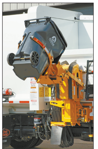
A demonstration of how the retractable arm on the new garbage trucks will reach out to grab and empty the new carts.
